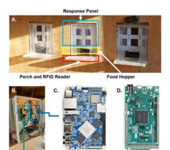
**Figure 3.** The response panels that face into the pigeon loft (A), behind the response panels is an LCD screen using to display stimuli (B), a NanoPC-T4 used to control the stimulus display (C) and an Arduino Due microcontroller that controls the administration of food (D).
