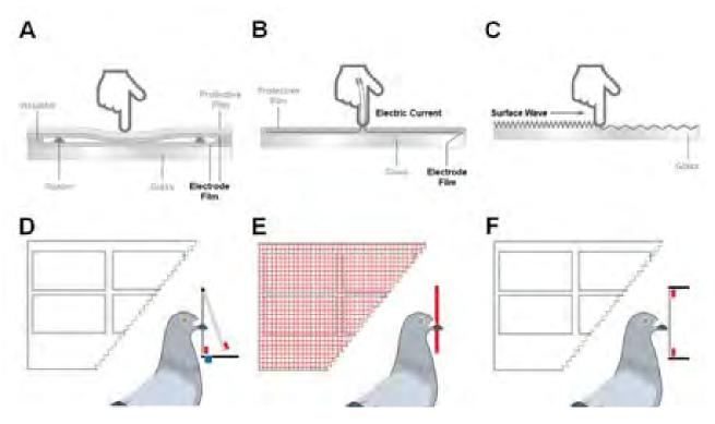
Figure 6. Resistive (A), capacitive (B), and acoustic wave touch screens (C). Flappy key (D), infra-red (E) and pressure sensitive (F) key setups.
